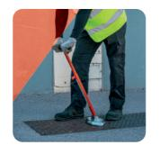
STEP 3 To take the magnet down, lower the handle against the unhooking stop
