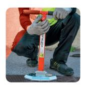
STEP 1 Adjust the handle using the adjustment button
